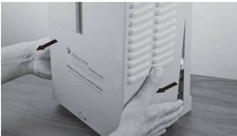
Figure 5 - Pull out bottom of cover
